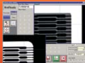
複雑な端子形状も正確に位置決め加工、 抜きずれ検査も可能 Advanced pattern recognition and cut position measurement
